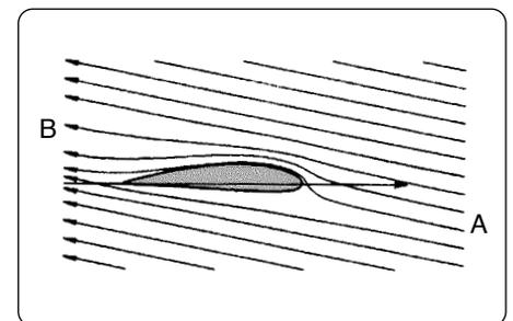
*Air flow around an aerodynamic profile*
